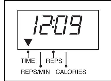
**Scan mode**—To select the scan mode, press the select button repeatedly until the scan mode indicator appears. The console will display the time, reps/min, reps, and calories modes in a repeating cycle. The mode arrows will show which mode is currently displayed.
