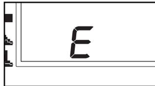
lower half of the display to show which unit of measurement is selected. To change the unit of measurement, first hold down the Program/Manual button for several seconds. An E (for English) or an M (for metric) will appear in the display. Press the Increase button to change the unit of measurement. When the desired unit of measurement is selected, press the Program/Manual button again. Note: When the batteries are replaced, it may be necessary to reselect the desired unit of measurement.
