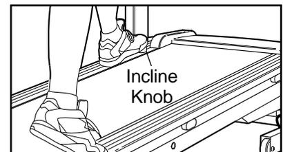
Using your left foot, press down the incline knob until the desired incline is reached. To decrease the incline, stand with your right foot near the front of the right foot rail while pressing down the incline knob. Note: It may be helpful to step off the treadmill when pressing down on the incline knob to decrease the incline.
