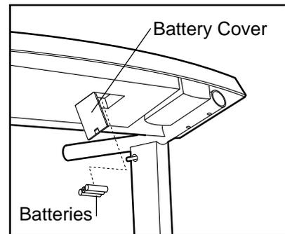
**Make sure that the negative ends of the batteries (marked “-”) are touching the springs in the battery compartment.** Close the battery cover.
