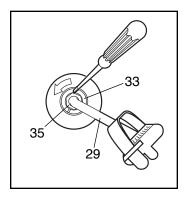
(33). Lightly tap the screwdriver with a hammer to turn the Slotted Bearing Nut counterclockwise until the arms are no longer loose. **Do not overtighten the Slotted Bearing Nut.** When the Slotted Bearing Nut is properly tightened, tighten the Crank Nut.
