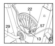
the Screw. Turn the Crank (29) for a moment. Repeat until the console displays correct feedback. When the
