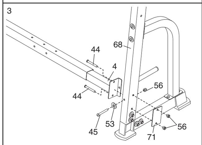
4. Attach the Crossbar (3) to the Right Upright (5) with two M10 x 72mm Button Screws (44), a Support Plate (71), an M10 x 93mm Button Bolt (45), an M10 Washer (53), and three M10 Nylon Locknuts (56). **Do not tighten the Locknuts yet.**
