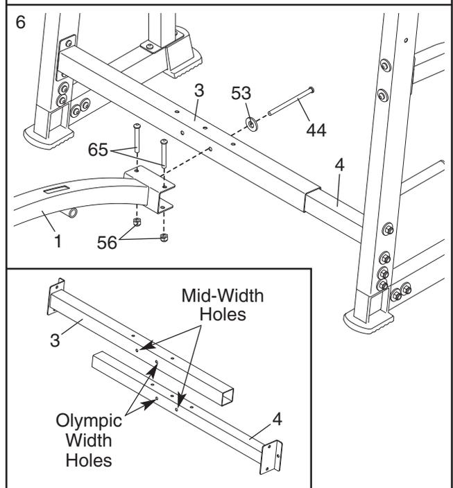
**Tighten the M10 Nylon Locknuts (56) and M10 Nylon Jamnuts (69) used in steps 1–6.**
