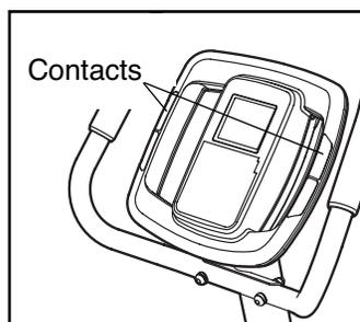
When your pulse is detected, one, two, or three dashes will appear in the display, and then your heart rate will be shown. For the most accurate heart rate reading, hold the contacts for at least 15 seconds. Note: If you continue to hold the handgrip pulse sensor, the display will show your heart rate for up to 30 seconds.
