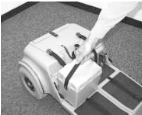
FIGURE 16. BATTERY REMOVAL / REPLACEMENT
