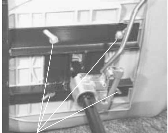
FIGURE 12. REMOVE THESE BOLTS TO ADJUST SEAT POSITION
