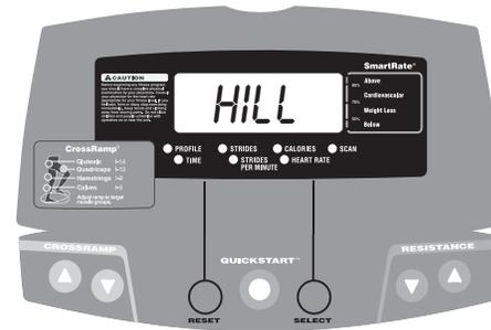
The resistance in the EFX5.19 Hill Climb program is preprogrammed. To override the resistance settings for each column, press the RESISTANCE arrow keys. The changes raise or lower the columns on the remaining portion of the program profile. Any changes you make are saved and applied the next time you use the Hill Climb program.
