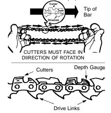
6. Place the chain over and behind the clutch, fitting the drive links in the clutch drum sprocket.
