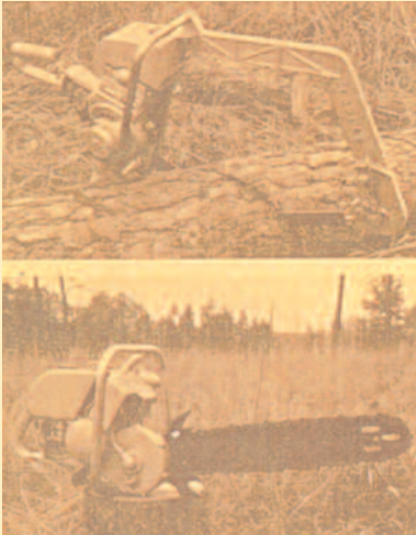
The Model A (top) was Poulan's first one-man bow saw offering Reduction Drive. The Model B100 (bottom) featured Gear Drive and led to dramatic growth of the company.
