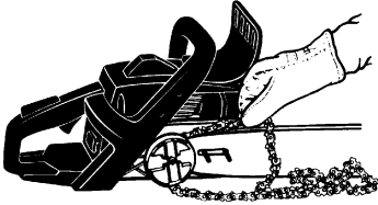
Place chain onto the sprocket
