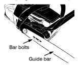
6. Carefully remove the chain from the package. Hold chain with the drive links as shown.
