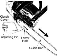
Install bar nuts and finger tighten only. Once the chain is tensioned, you will need to tighten bar nuts.
