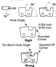
AWARNING: Maintain the proper hook angle according to the manufacturer's specifications for the chain you are using. Improper hook angle will increase the chance of kickback which can result in serious injury.
