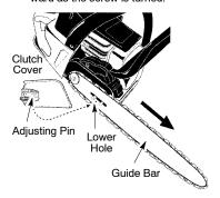
12. Install bar nuts and finger tighten only. Once the chain is tensioned, you will need to tighten bar nuts.
