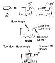
**AWARNING:** Maintain the proper hook angle according to the manufacturer's specifications for the chain you are using. Improper hook angle will increase the chance of kickback which can result in serious injury.
