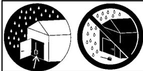
Store unit indoors in a high, dry place out of the reach of children. Store unit and fuel in area where fuel vapors cannot reach sparks or open flames from water heaters, electric motors or switches, furnaces, etc.
