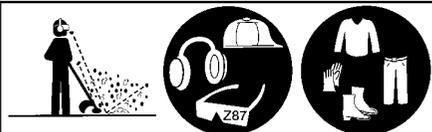
Blade/trimmer line can throw objects violently. You can be blinded or injured. Always wear hearing protection and safety glasses marked Z87. Always wear head protection, heavy, long pants, long sleeves, boots and gloves.
