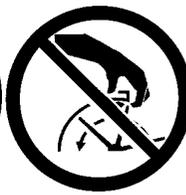
**⚠ WARNING:** Never lean over discharge chute. Rocks or debris could be thrown into the eyes and face and cause serious injury or blindness.
