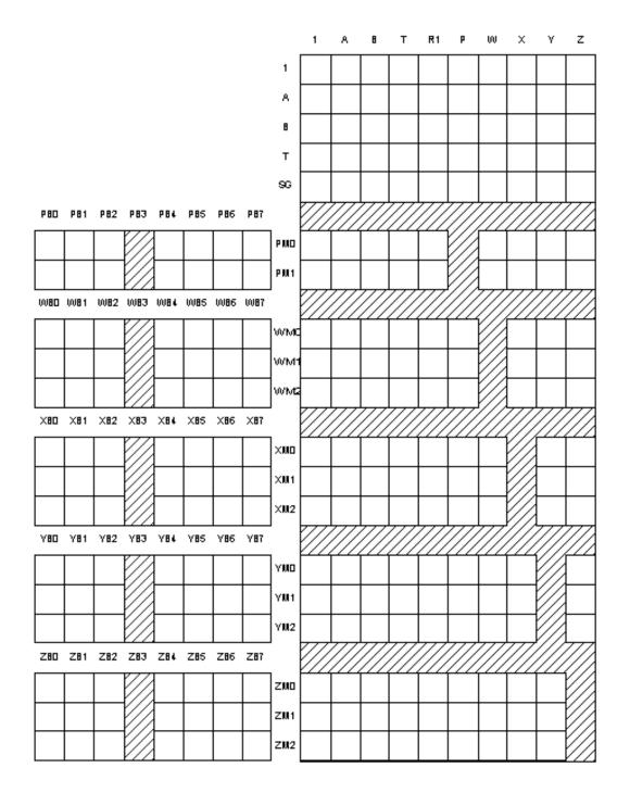
The EF2211 has three analog outputs labeled 1, A, and B. These outputs are all at line level. There are two additional outputs: the output to the telephone interface, labeled T, and the output to the power amplifier. The output to the power amplifier does not have a separate output in the matrix, it is
