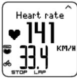
Press and hold UP to zoom into the upper row, and DOWN to zoom into the middle row. Return to the normal display by pressing and holding the button again.
