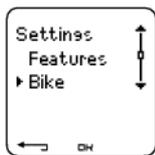
Select **Settings > Bike > Bike 1, Bike 2, Bike 3** or **Other**. Bike 2 and Bike 3 can be turned on or off. Select **Other** to deactivate speed, cadence and power sensors, and to measure heart rate, altitude, and temperature data only.
