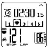
If, for example, you are cycling with a heart rate of 130 bpm which is 75% of your maximum heart rate, and matches sport zone 3, you can press and hold LAP to lock your heart rate into this zone. **Sport zone3 Locked 70-79** is displayed. An alarm sounds if you are below or above the sport zone (if the target zone alarm function is on). Unlock the sport zone by pressing and holding OK again: **Sport zone3 Unlocked** is displayed.
