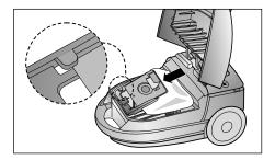
4) Press the dust cover down gently until the clamper relocks.
