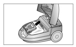
After removing the used dust bag, insert the cardboard bag collar of the new dust bag into the suction inlet to the full.
