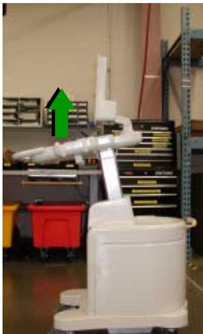
Figure 10-54 Raising the Control Panel
