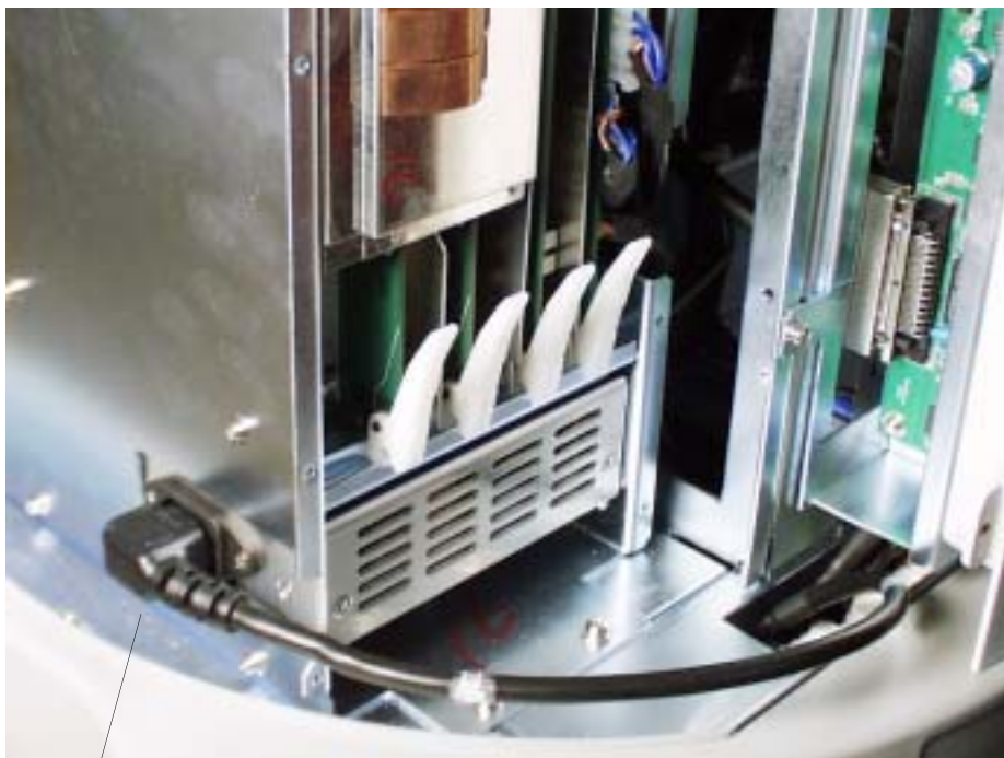
Figure 10-26 Disconnecting the Power Supply Power Cord
