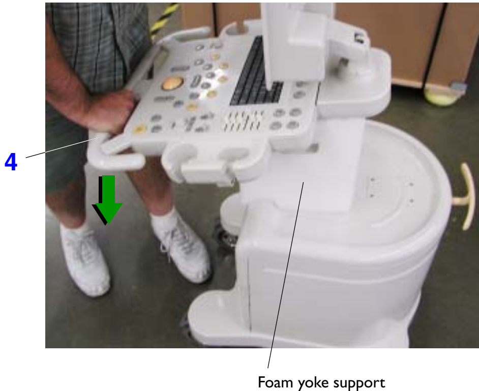
Figure 10-56 Lowering the Control Panel
