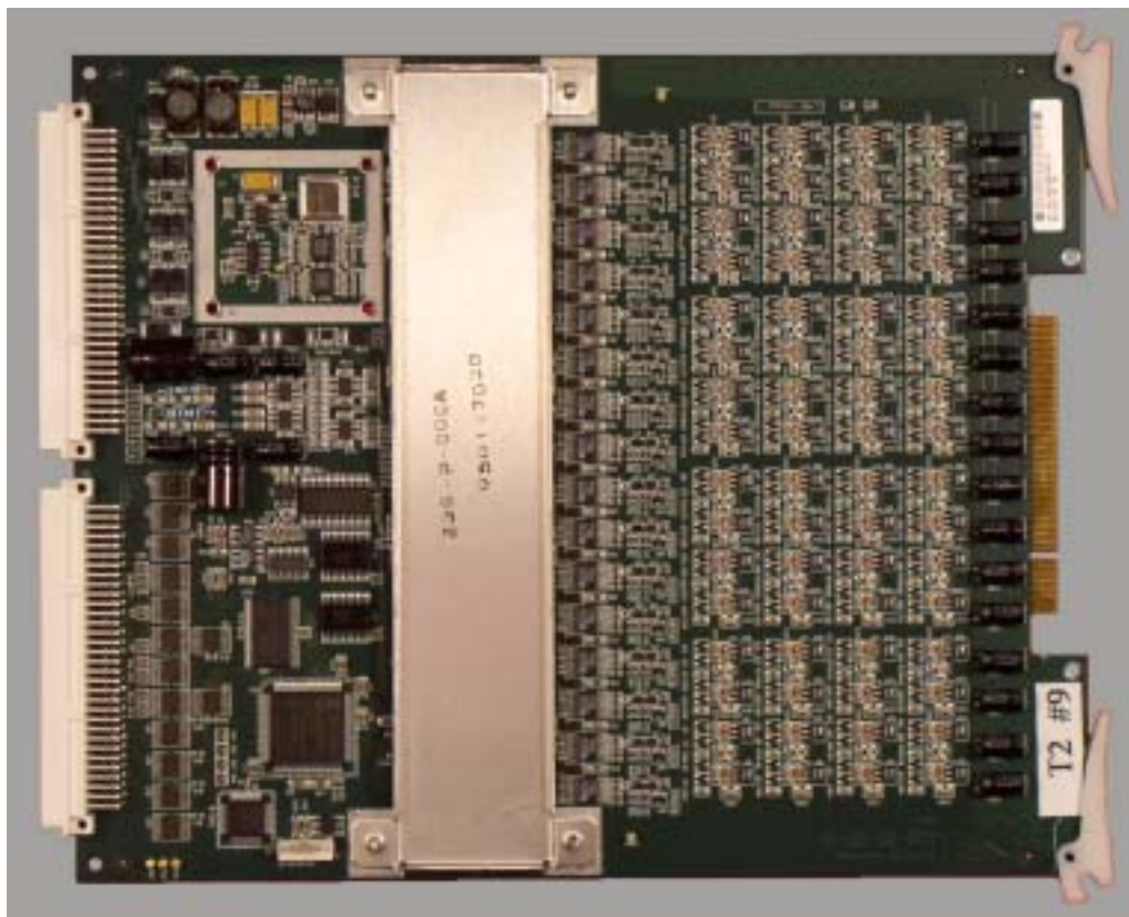
Figure I3-12 Beamformer (BF) Board
