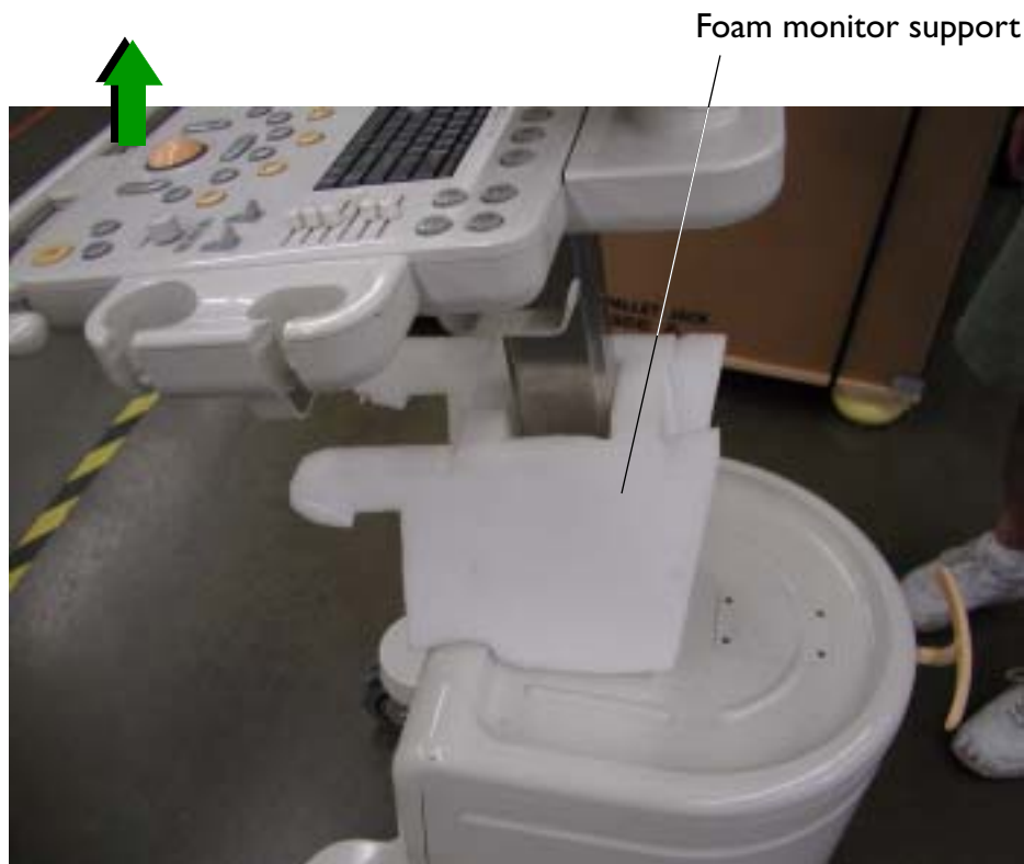
Figure 5-12 Removing the Shipping Materials (Yoke Support)
