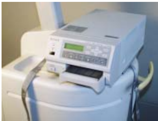
Figure 5-21 Placing and Strapping the Color Printer to the Universal Peripheral Mounting Plate
