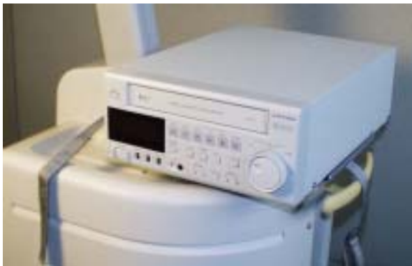
Figure 5-27 Placing and Strapping the VCR to the Universal Peripheral Mounting Plate
