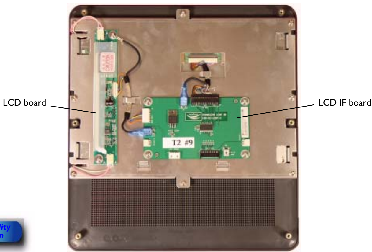
Figure I3-5 Video Monitor PCBs (Back of Monitor LCD)
