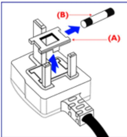
If the mains plug contains a fuse, this should have a value of 5A. If a plug without a fuse is used, the fuse at the distribution board should not be greater than 5A.
