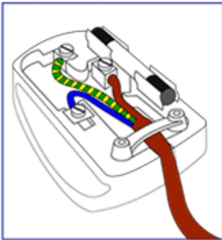
2. The BLUE wire must be connected to the terminal which is marked with the letter "N" or coloured BLACK.
