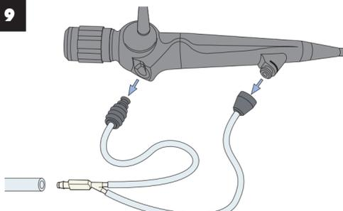
Turn the suction pump off. Hold the control section with the openings pointing down and disconnect the suction cleaning adapter.
