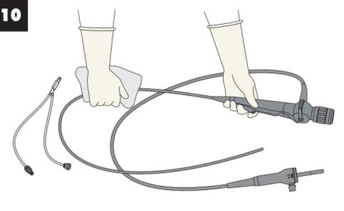
Dry the bronchoscope and adapter with an alcohol-moistened cloth. Make sure that the equipment is completely dry prior to storage.
