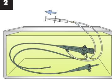
Attach a syringe to the adapter. Pull the plunger of the syringe to fill the instrument/suction channels and channel cleaning adapter with disinfectant solution.
