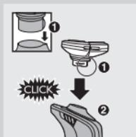
**2** Insert the lug of the new shaving unit into the slot in the top of the shaver (1). Then press the shaving unit downwards (2) to attach it to the shaver ('click').
