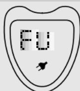
► As soon as the battery has been fully charged, the plug symbol appears and the word 'FULL' runs across the display every 9 seconds.
