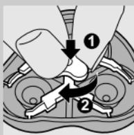
**4** Remove the shaving heads and place new ones in the shaving unit in such a way that the parts with the small holes point towards the centre of the shaving unit.
