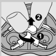
**2** Press the release button (1) and open the shaving unit (2).
