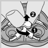
**1** Open the shaving unit, turn the wheel anticlockwise (1) and remove the retaining frame (2).
