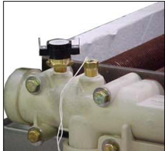
5. Remove the 8 bolts holding the main inlet/outlet head.
