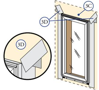
D. **Apply flashing tape to diagonal cuts.** Cut pieces of flashing tape at least 1" longer than the diagonal cuts in the water resistive barrier. Apply the tape covering the entire diagonal cut in the water resistive barrier at both upper corners of the window.
