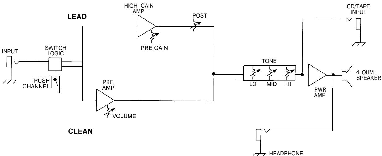
This block diagram shows signal flow within the unit. In order to thoroughly understand the unit's functions, please study the block diagram carefully.
