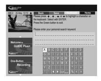
Use the ↑/\$/←/→ buttons followed by ENTER to select characters from the on-screen keyboard. When you're finished, press the GREEN Action button to exit and continue.
