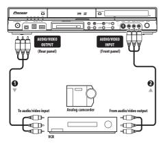
1 Connect a set of audio and video inputs of your VCR or camcorder to a set of outputs on this recorder.
