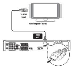
The arrow on the cable connector body should be face down for correct alignment with the connector on the recorder.
