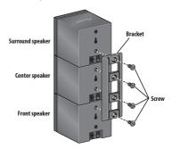
When placing the center speakers independently, stack the front speaker on the bottom and the surround speaker on top, then align the 1st and 3rd screw holes from the top of the bracket with the upper screw holes on the back of the speakers, and fasten the two securely.
