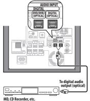
Connect the DVD/DVR2 (OPTICAL) or DIGITAL (OPTICAL) jack on the rear panel to the optical output of an external playback component.
