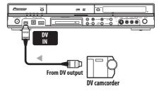
Use a DV cable (not supplied) to connect the DV jack of your DV camcorder to the front panel DV IN jack of this recorder.
