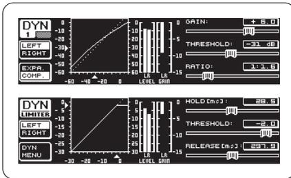
Everything you'd find on a dedicated compressor/expander is here including variable ratios from 1:1.1 to 1:100, ATTACK times from 0 to 200ms, 0-3dB variable knee and 20 to 4000ms RELEASE, all adjustable from a coarse/fine adjustment scale. The built-in separate LIMITER has Threshold, Hold and Release functions.
