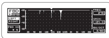
With the digital capabilities we've just listed, it's easy to see why we were able to include a highly-effective Feedback Destroyer (FBD) feature — it's essentially a dynamically-activated parametric EQ that “watches” the whole frequency spectrum in 1/60-octave bands and then instantly identifies and notches out feedback.
