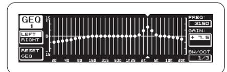
Naturally the DEQ2496 has phase-neutral digital graphic EQ...but in addition we've added a function that allows you to change the bandwidth of each frequency from standard 1/3 to as much as 59/3.
