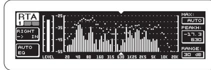
The DEQ2496 features an FFT real time analyzer for precise graphic display of 61 frequency bands. You can monitor main or digital inputs and outputs, AUX/digital out or a feed from an RTA microphone and display the results in a multitude of ways including funky retro VU meters.
