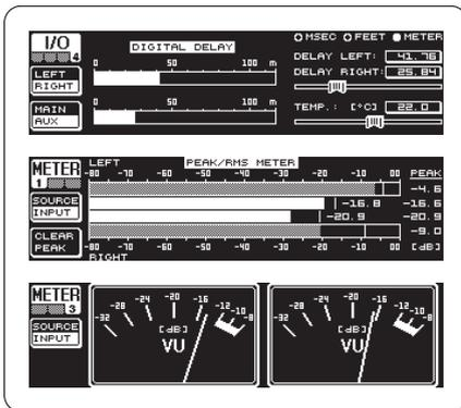
Not only can you specify time delay in feet or meters but simultaneously compensate for ambient temperature which affects sound speed!
