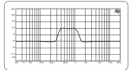
Graphic equalizer with frequency response correction (TRUE RESPONSE)
