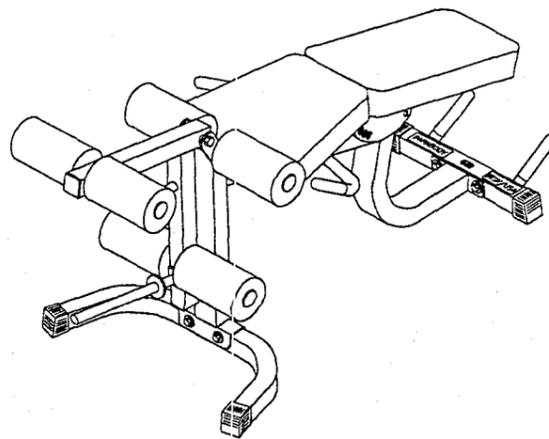
**STEP 1:** Insert four PARABODY LOGO END CAPS (37) into the ends of REAR BASE LEG (12) and FRONT BASE SUPPORT (1). See FIGURE 1.
