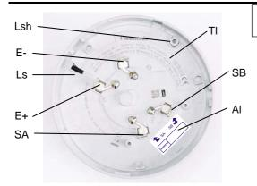
The detector is plugged in the analog base 3312x / 4313. The COM loop / Ext. LED are connected to the analog base.
