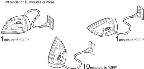
NOTE: 1. The Auto shut off system works regardless of position of the temperature selector dial, even at "OFF" position.
