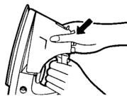
5 The water level can be observed through the transparent part of the tank, when iron is placed either horizontally or vertically. When the water level becomes low, place the iron vertically and add water, following the procedure described in 1 to 4 above.
