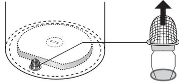
The filter can be removed by pulling firmly on it.
