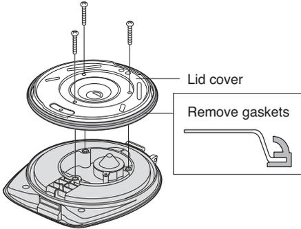
Remove lid, unscrew 3 tapping screws and remove the lid cover.
