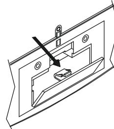
3.) Insert 2 "AA" alkaline batteries into the compartment as illustrated.
