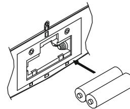
4.) Replace the battery door and place the radio right side up.
