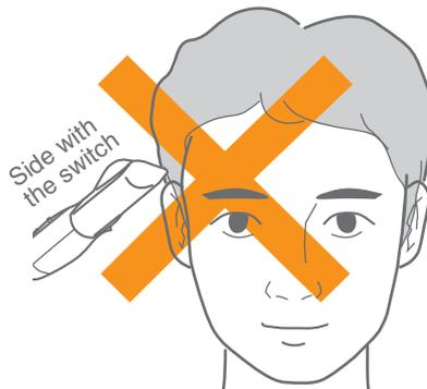
Do not use the trimmer switch side up as shown in the illustration on the left. This will result in cutting more than the desired length.
