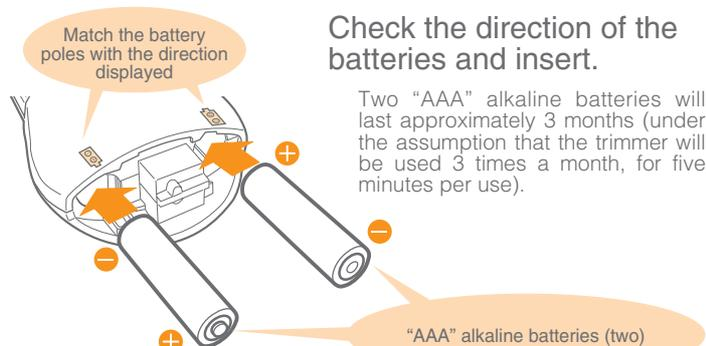
Check the direction of the batteries and insert.
