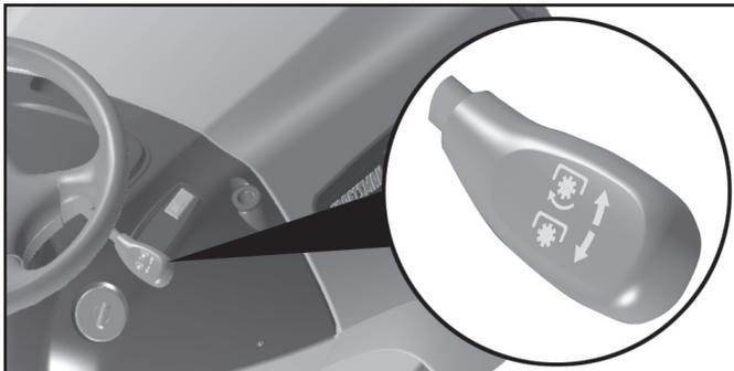
(☒) ATTACHMENT CLUTCH LEVER “DISENGAGED”
