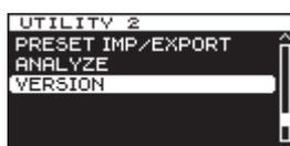
2. Press the **MULTI JOG** dial to open the VERSION screen. The VERSION screen shows information about the firmware version and build number.
