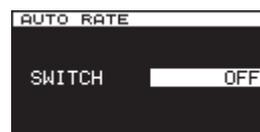
3. Turn the **MULTI JOG** dial to turn the automatic video frame rate setting function on or off.
