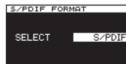
3. Turn the **MULTI JOG** dial to set the output format for the **S/PDIF 1/2 OUTPUTS** (RCA pin jacks).
