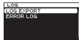
2. Press the **MULTI JOG** dial to open the ERROR LOG screen. In the error log, each error is shown on a separate page.
