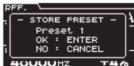
3. Press the **MULTI JOG** dial to save the unit's current settings to the **PRESET** that you pressed in step 2.
