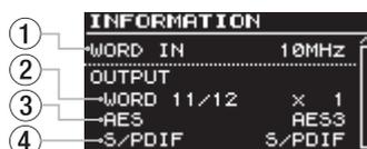
Example of display when reference redundancy function is on
