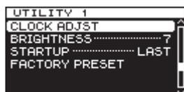
2. Press the **MULTI JOG** dial to open the **CLOCK ADJUST** screen.
