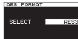
3. Turn the **MULTI JOG** dial to set the output format for the **AES 3/11 1/2 OUTPUTS** (balanced XLR).
