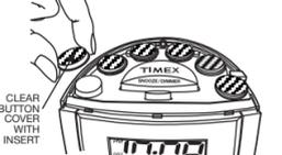
Replace the clear cover together with paper insert on the top of black button.
