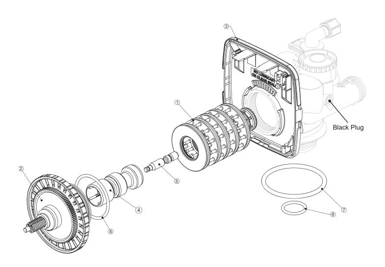
WS1.25EI Drive Cap Assembly, Downflow Piston, Regenerant Piston and Spacer Stack Assembly
