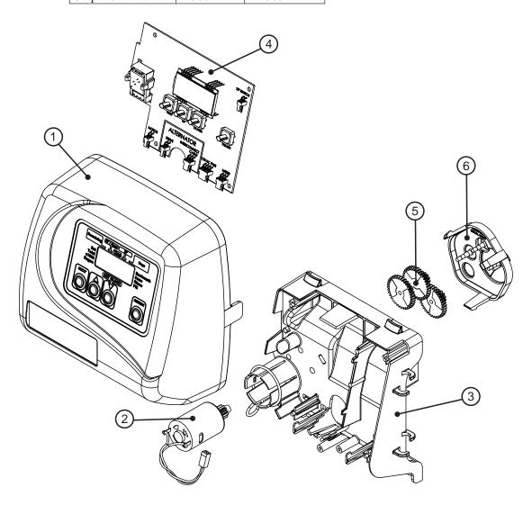
WS1EI Drive Cap Assembly, Downflow Piston, Regenerant Piston and Spacer Stack Assembly
