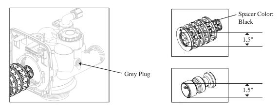
WS1.25 with 32mm Distributor Tube Opening Identification
