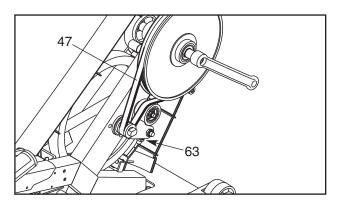
Next, turn the indicated M10 Nylon Locknut (63) until the Drive Belt (47) is properly tightened. Then, reattach the right side shield.
