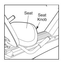
seat knob snaps into one of the holes in the seat rail.
