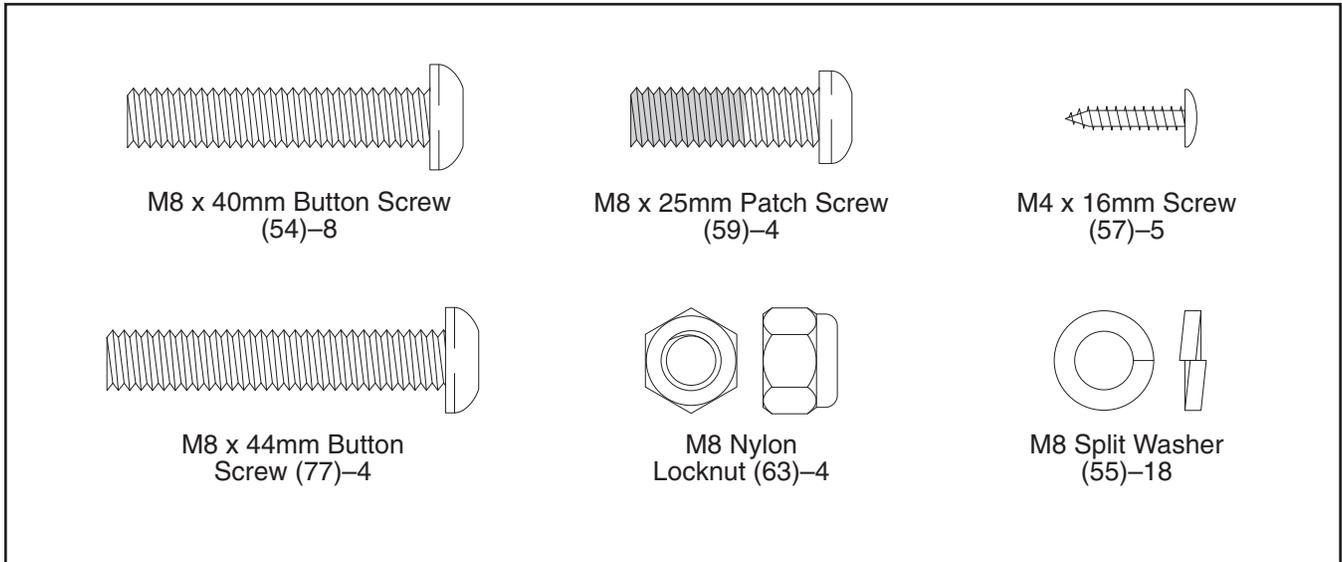
1. Identify the Front Stabilizer (15). While another person lifts the front of the Frame (1), attach the Front Stabilizer to the Frame with four M8 x 40mm Button Screws (54) and four M8 Split Washers (55).
