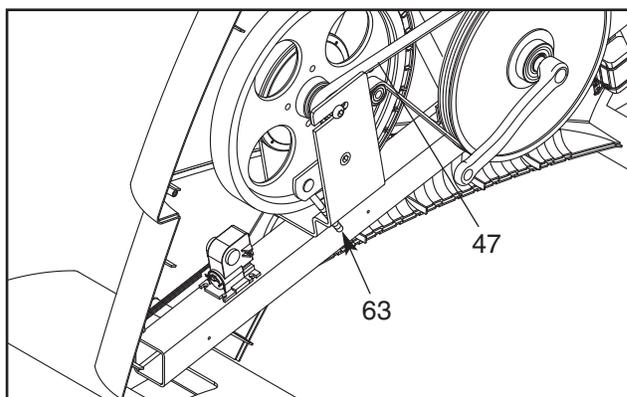
Next, turn the indicated M8 Nylon Locknut (63) until the Drive Belt (47) is properly tightened. Then, reattach the side shields.
