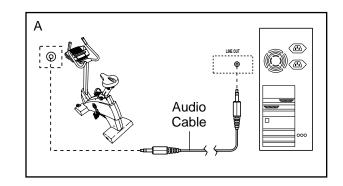
B. Plug one end of the audio cable into the jack beneath the console. Plug the other end of the cable into a 1/8" Y-adapter (available at electronics stores). Plug the Y-adapter into the PHONES jack on your computer. Plug your headphones or speakers into the other side of the Y-adapter.
