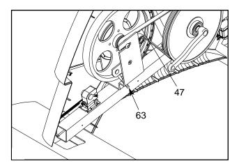
Next, turn the indicated M8 Nylon Locknut (63) until the Drive Belt (47) is properly tightened. Then, reattach the side shields.
