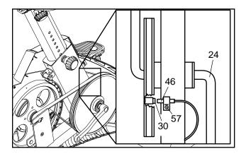
Turn the right crank arm for a moment. Repeat until the console displays correct feedback. When the reed switch is correctly adjusted, reattach the right side shield and the right pedal.
