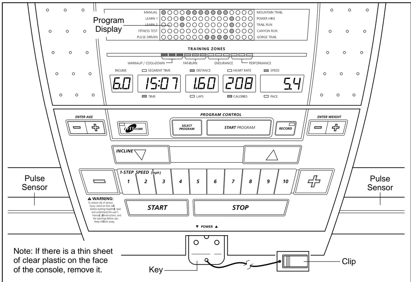
Note: If there is a thin sheet of clear plastic on the face of the console, remove it.
