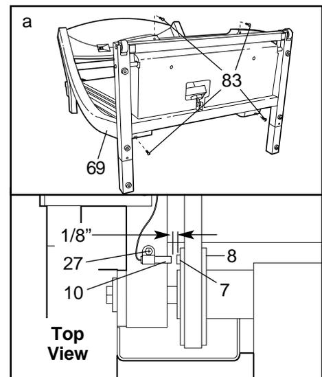
Locate the Reed Switch (10) and the Magnet (7) on the left side of the Pulley (8). Turn the Pulley until the Magnet is aligned with the Reed Switch. **Make sure that the gap between the Magnet and the Reed Switch is about 1/8"**. If necessary, loosen the Screw (27) and move the Reed Switch slightly. Retighten the Screw. Re-attach the hood, and run the treadmill for a few minutes to check for a correct speed reading.
