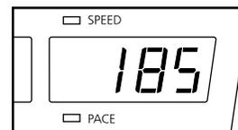
To enter your weight, press either of the Enter Weight buttons. The current weight setting will appear in the Speed/Pace display. Press the Enter Weight buttons again to enter your weight. Four seconds after the buttons are pressed, the weight setting will disappear from the display. Your weight will then be saved in memory.
