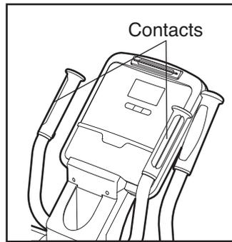
When your pulse is detected, your heart rate will be shown in the display. For the most accurate heart rate reading, hold the contacts for at least 15 seconds.
