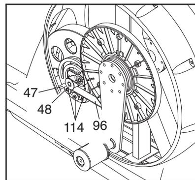
Reattach the left disc with the four screws and then reattach the left disc cover.
