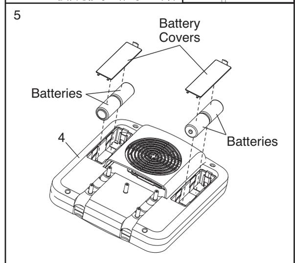
Note: The Console (4) can be operated with an optional power supply instead of batteries. **To purchase a power supply, call the toll-free telephone number on the front cover of this manual.** Plug one end of the power supply into the jack at the front of the exercise cycle. Plug the other end of the power supply into an appropriate outlet that is properly installed in accordance with all local codes and ordinances.
