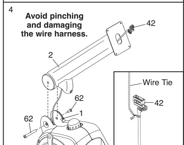
Attach the Upright (2) to the Frame (1) with an M10 x 63mm Bolt Set (62). **Be careful to avoid pinching the Upper Wire Harness (42).**
