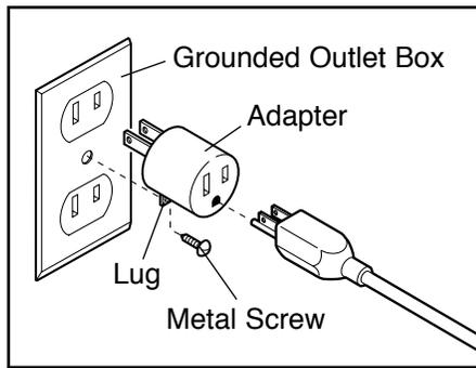
The green-colored rigid ear, lug, or the like extending from the adapter must be connected to a permanent ground such as a properly grounded outlet box cover. Whenever the adapter is used, it must be held in place by a metal screw. **Some 2-pole receptacle outlet box covers are not grounded. Contact a qualified electrician to determine if the outlet box cover is grounded before using an adapter.**
