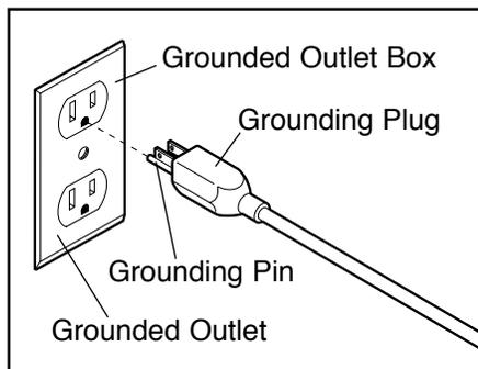
erly installed and grounded in accordance with all local codes and ordinances. This product is for use on a nominal 120-volt circuit. **Important: The elliptical crosstrainer is not compatible with GFCI-equipped outlets.**
