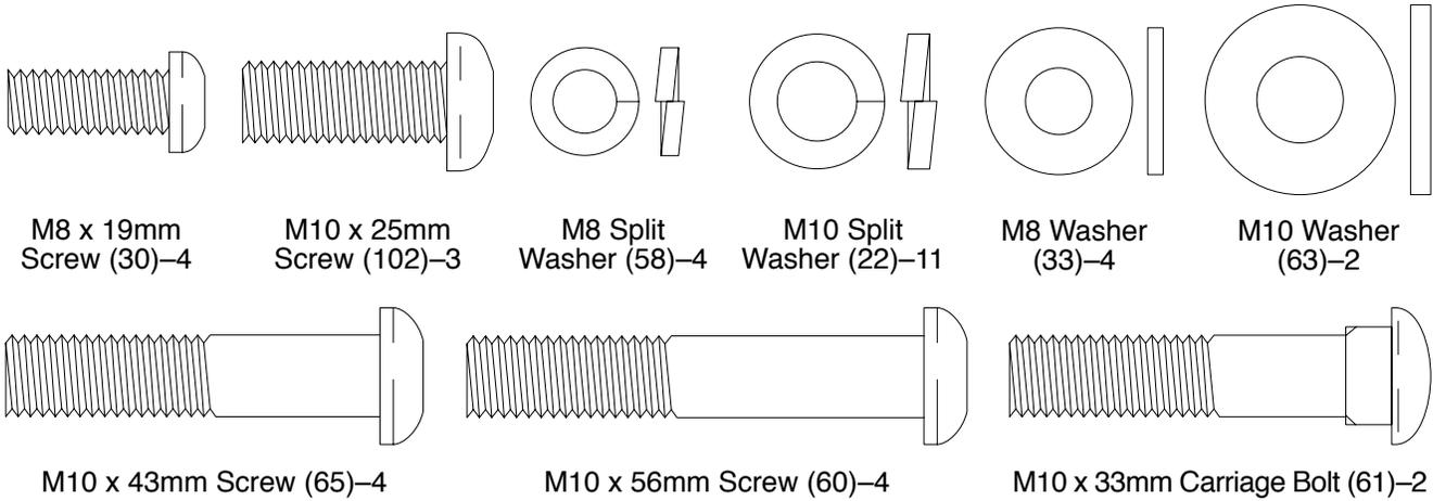
1. Identify the Rear Stabilizer (59), which has Leveling Feet (14) threaded into it. Attach the Rear Stabilizer to the Frame with the four M10 x 56mm Screws (60) and four M10 Split Washers (22).
