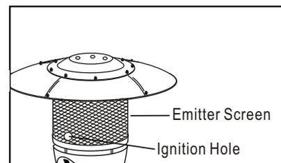
**CAUTION :** Avoid inhaling fumes emitted from the heater's first use. Smoke and odor from the burning of oils used in manufacturing will appear. Both smoke and odor will dissipate after approximately 30 minutes. The heater should NOT produce thick black smoke.
