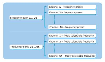
Each of the channels in the frequency banks "1" to "20" has been factorypreset to a fixed frequency (frequency preset). The factory-preset frequencies within one frequency bank are intermodulation-free. These frequencies cannot be changed.
