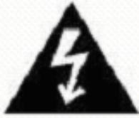
The Lightning flash with arrowhead symbol, with an equilateral triangle is intended to alert the user of the presence of uninsulated dangerous voltage within the product's enclosure that may be of sufficient magnitude to constitute a risk of electric shock to persons.
